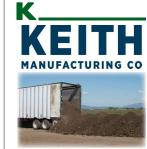
Keith Mfg Co (541) 475-3802 sales@keithwalkingfloor.com www.keithwalkingfloor.com The KEITH® WALKING FLOOR® system is a horizontal unloader installed in a trailer, that "walks" material out of the trailer with no tipping. Unload in areas inaccessible to dump or tipping inaccessible to dump or tipping and trees or inside buildings. See ad on pg 25
